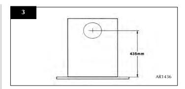
6.2 A 152mm (6') diameter hole is required to install the flue. This can be achieved by either:a) Core drill
